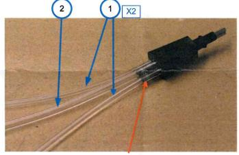
Inspect tubing, over metal tubes of probe tip, for damage. If damage is visible, check inside of metal tubing for blockage.
